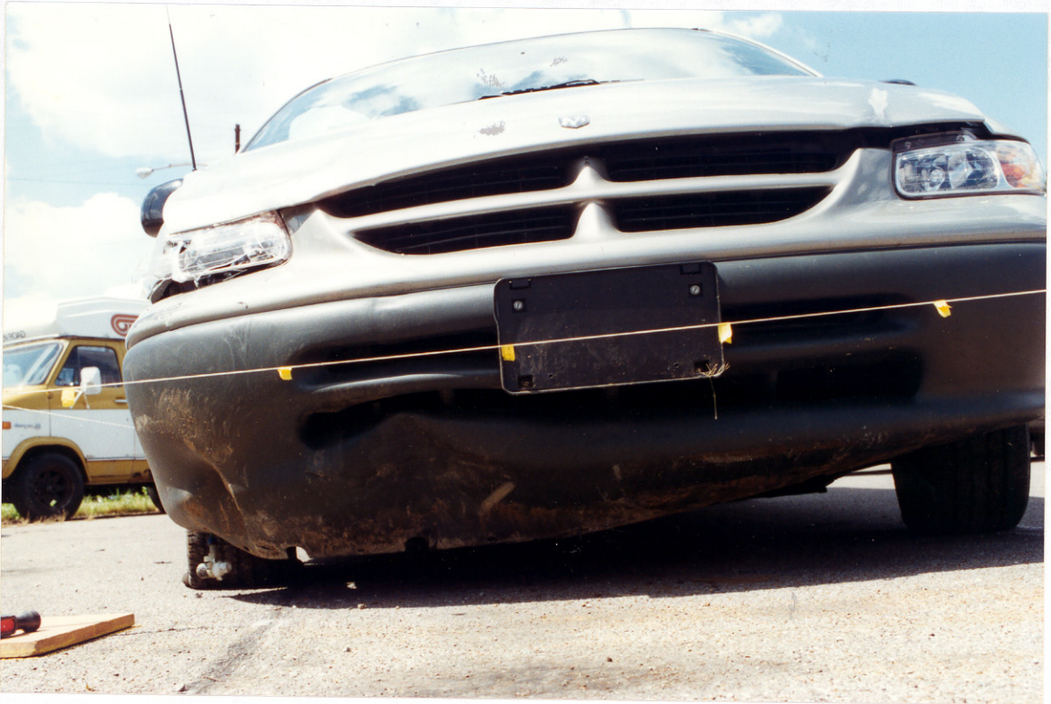
34. Front view of the damage to the lower surface of the bumper fascia.
